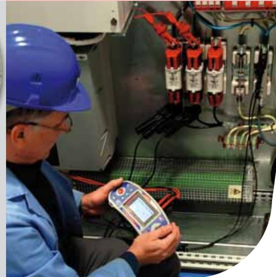
**MI 2230 VAFMeter is handheld multifunction instrument which can accurately measure voltage, current, power, harmonic distortion and phase angles in single, two and three phase systems.**
