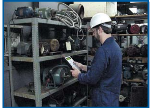
Testing spare motors to confirm their status insures against installing a faulty motor.
