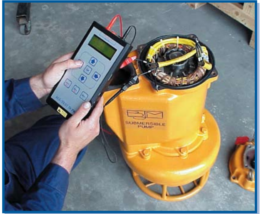
Testing the electrical health of a motor/pump combination lets you make a better repair/replace decision.
